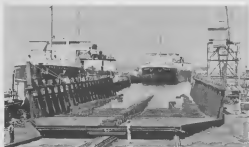
Lago's Drydock where Lake tankers were regularly hauled ashore for repairs or maintenance.
